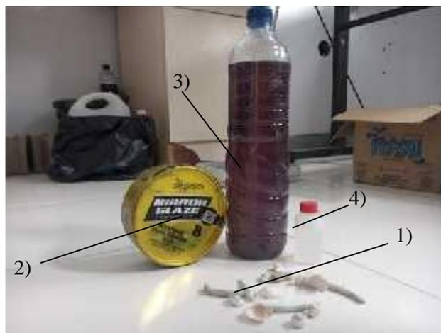
Figure 1. Working materials used to make flooring material from shellfish (Source: Author collections, 2017)
