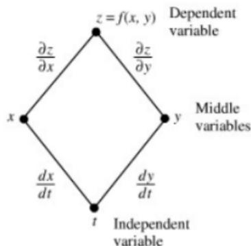
$$\frac{dz}{dt} = \frac{\partial z}{\partial x} \frac{dx}{dt} + \frac{\partial z}{\partial y} \frac{dy}{dt}$$
