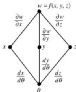
$$\frac{dw}{d\theta} = \frac{\partial w}{\partial x} \frac{dx}{d\theta} + \frac{\partial w}{\partial y} \frac{dy}{d\theta} + \frac{\partial w}{\partial z} \frac{dz}{d\theta}$$
