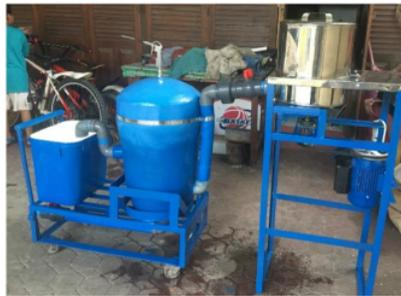
Gambar 11. Reaktor Gas Tipe Fixed Dome
