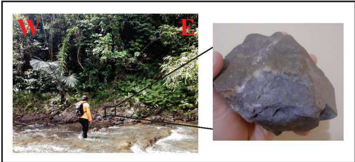
Figure 3. Outcrop of altered andesite units at the study site and hand specimen of altered andesite rock samples
