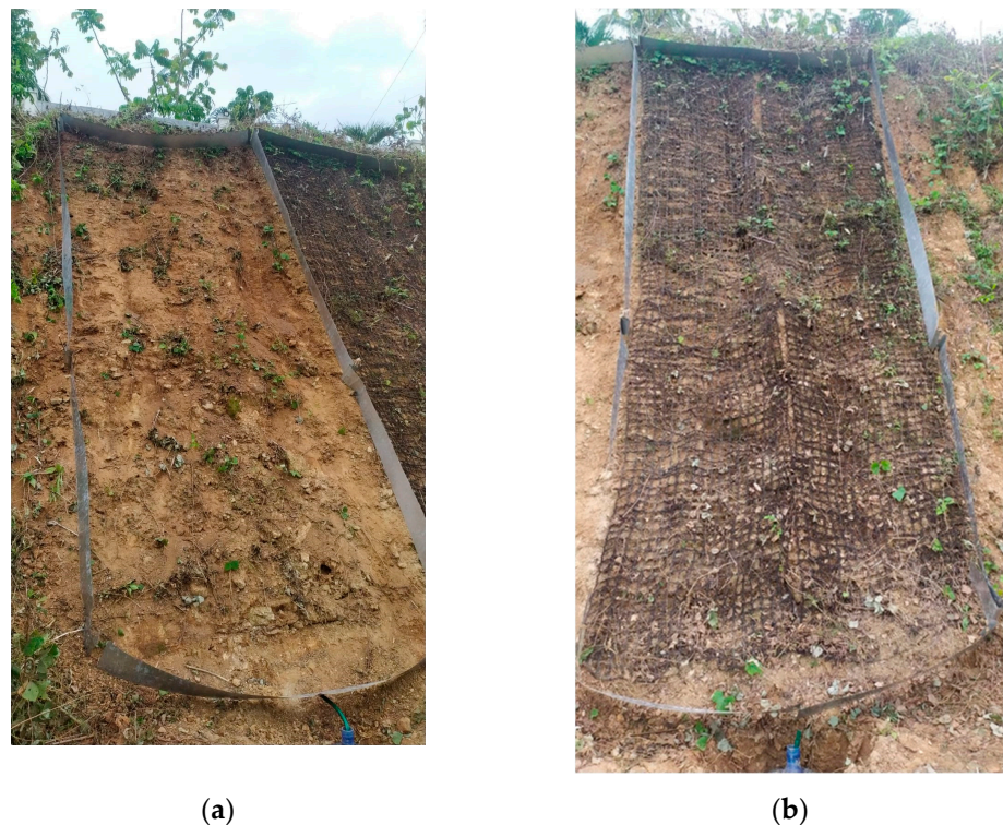
Figure 5. Design of field experiment on bare-soil plot (a) and ECB-covered plot (b); metal plate borders are installed to avoid eroded soils from falling outside the designed collectors placed below.
