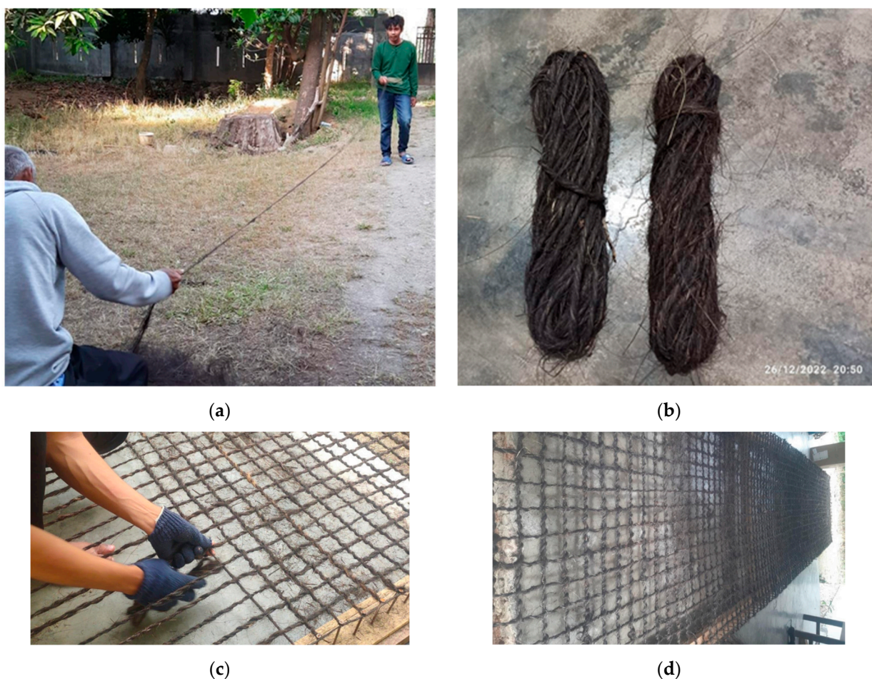
Figure 2. A sugar-palm-fiber-based net being prepared from previously manufactured (a) sugar palm fiber ropes with a diameter of 6 mm (b), woven on top of a nailed wooden frame (c); (d) the completed product.
