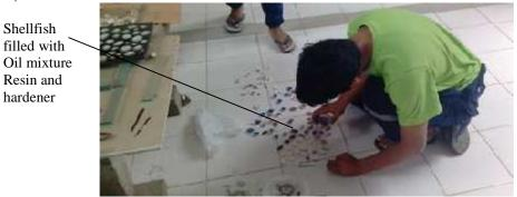
Figure 2. Fan shaped shells filled with a mixture of resin and hardener oils (Source: Author Collections, 2017).
