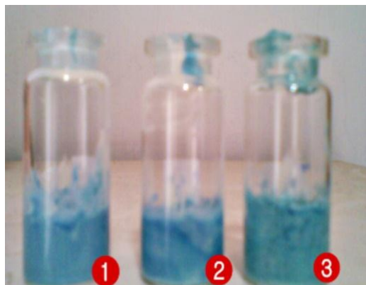
Fig. 2 Emulsion type test with color dispersion method
