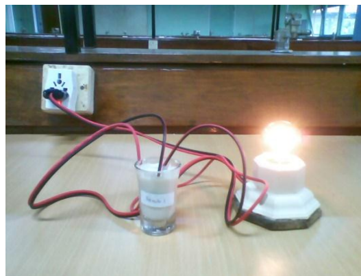
Fig. 3 Emulsion type test with electrical conductivity method
