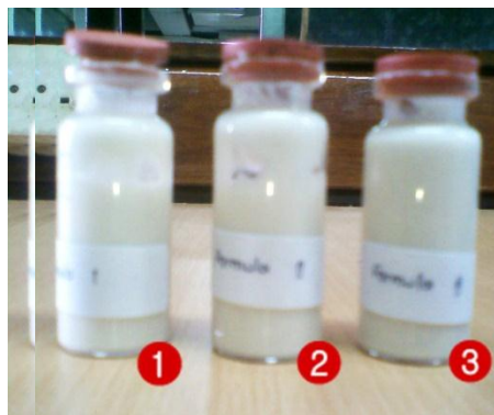
Fig. 1 Emulsion type test with dilution method
