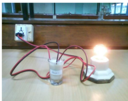
Fig. 3 Emulsion type test with electrical conductivity method
