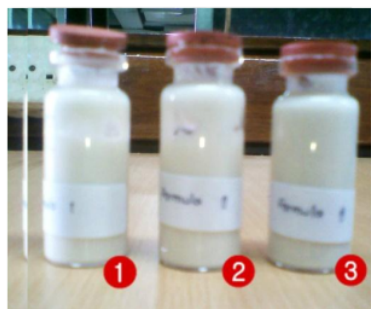
Fig. 1 Emulsion type test with dilution method
