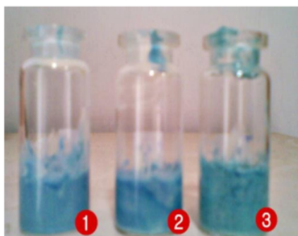
Fig. 2 Emulsion type test with color dispersion method
