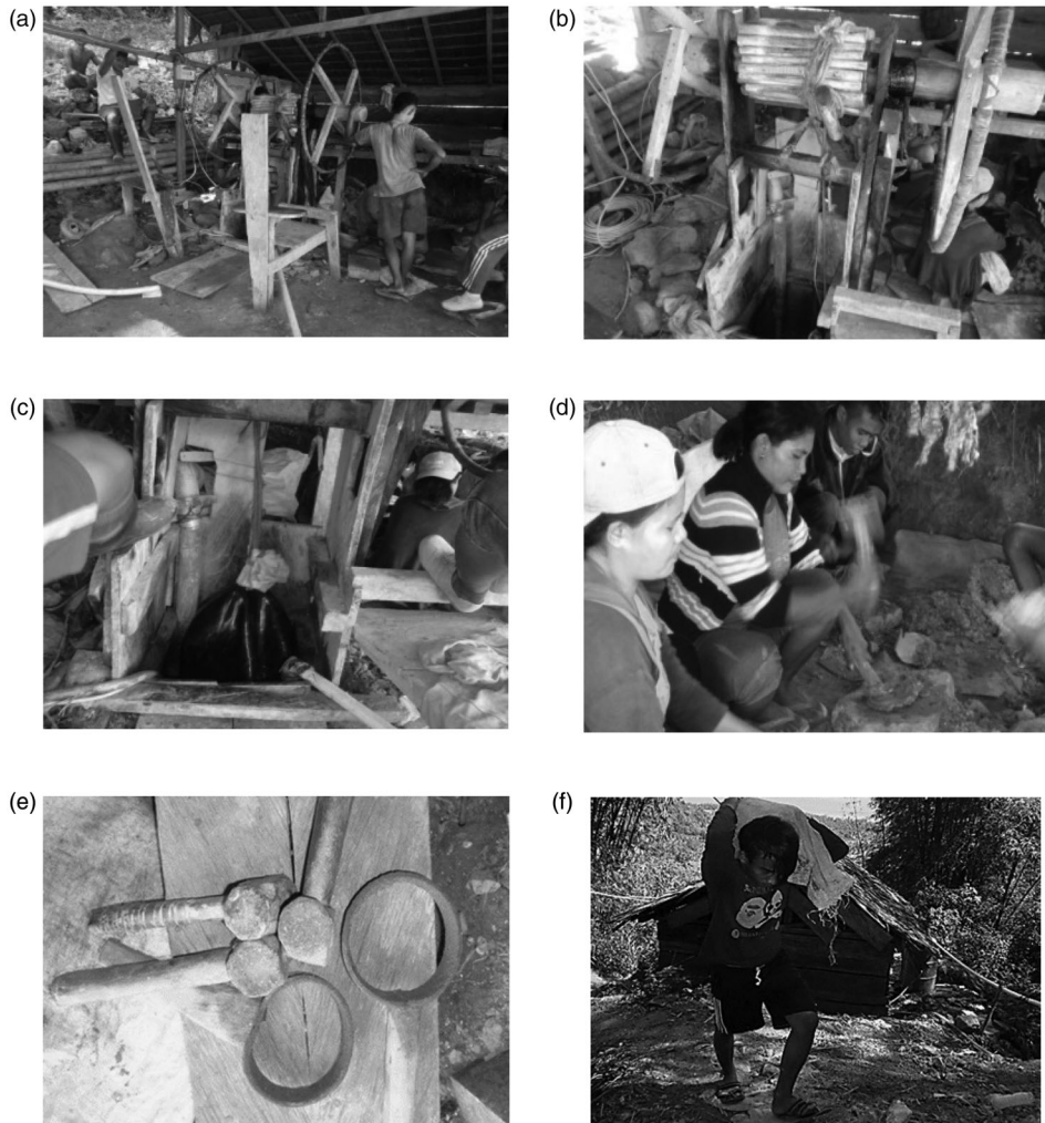
Figure 3. ASGM in the Gorontalo Utara Regency: (a) An artisanal mine shaft on a slope. (b) A hole where the miners are working. (c) A sack of ore is being pulled from the base of the hole. (d) The ore is manually crushed using simple tools. (e) The percussion tools used to crush the ore. (f) Raw crushed ore is manually transported to the processing plant.
