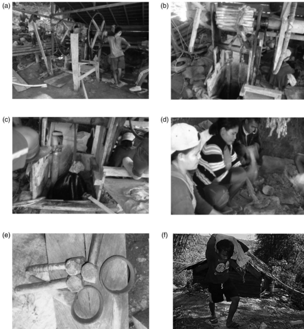
Figure 3. ASGM in the Gorontalo Utara Regency: (a) An artisanal mine shaft on a slope. (b) A hole where the miners are working. (c) A sack of ore is being pulled from the base of the hole. (d) The ore is manually crushed using simple tools. (e) The percussion tools used to crush the ore. (f) Raw crushed ore is manually transported to the processing plant.
