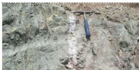
Figure 5. Carbonate vein in diorite (photo direction N 40° E).
