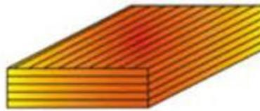
*Gambar 2. 4 Continous fiber composite (Gibson ,1994)*
