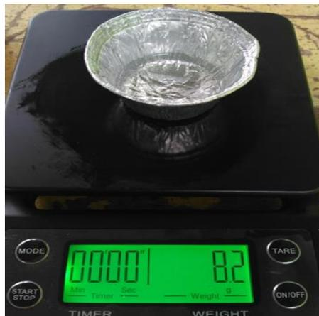
*Gambar 3. 24 Penimbangan clear epoxy resin hardener*
