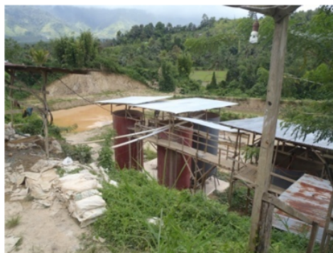
Figure 2. The Cyanidation plant in Tobongon, three cylinders left and four cylinders right and pond of mining waste is behind.
