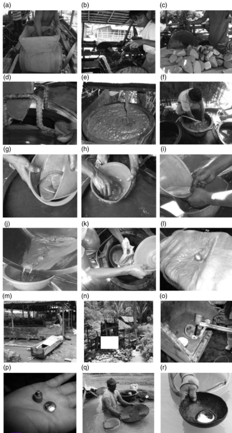
**Figure 4.** Artisanal and Small-scale mining (ASGM) activities in three locations in the Gorontalo Utara Regency. (a) Crushed ore is inserted into the ball mill (b) Water is poured into the trommel (c) The softball size rocks used to mill the ore inside the trommel (d) Where mercury is poured into the trommel mill (e) Discharging the trommel. (f) Separating
