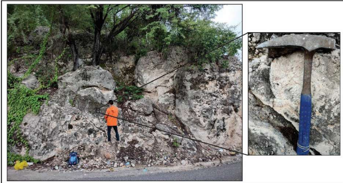
Figure 2. Coral limestone outcrops located in the hills of the southern part of Gorontalo Province
