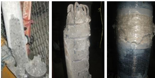
(a) Specimen PS (b) Specimen BT (c) Spec. B-1 LS Fig. 5. Models of failure of specimens 1, 2, 3
