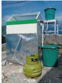
Gambar 6. Alat filter air laut
